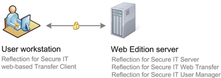
A typical distributed configuration is shown below. This configuration supports file exchange between users outside the network and a file server behind the firewall. It also puts the User Manager behind the firewall.
